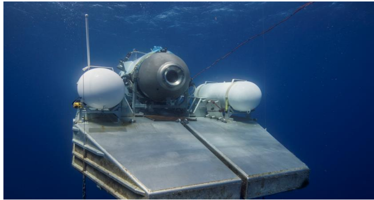
TITAN mounted on Launch and Recovery System
