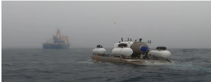
TITAN submersible with Launch and Recovery System in tow behind the Polar Prince
