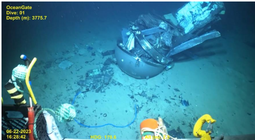
Rear Titanium hemisphere and carbon fiber pressure vessel as found on ocean floor
