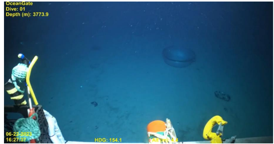
Front titanium hemisphere, as found on ocean floor
