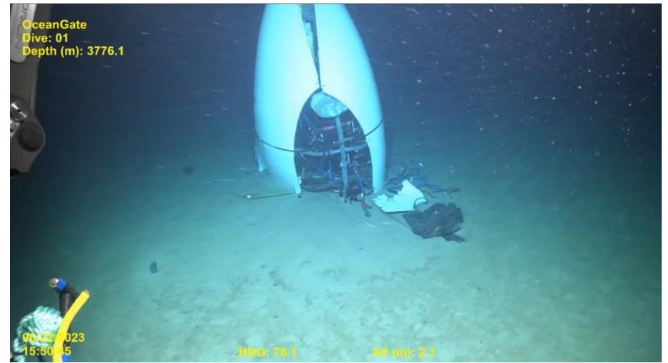
Rear fairing, as found on seafloor at 3776M deep near titanic wreckage
